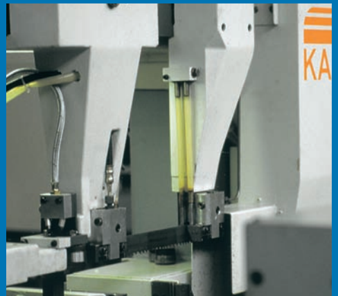
Sawing head with 2 nozzles on KASTO ribbon saws (band height 41 mm respectively)
