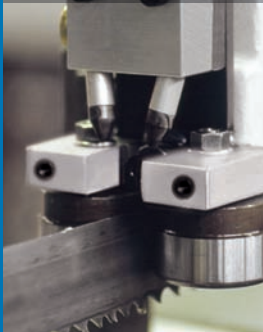
Sawing head with 2 nozzles on KASTO ribbon saws (band height 41 mm respectively)
