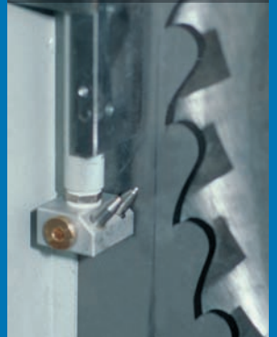
Nozzle head with two nozzles on circular saw (diameter of circular saw blade > 700 mm)
